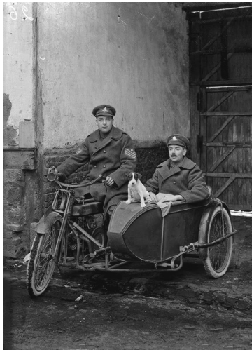
Douglas 4 HP (600cc) SV motorcycle combination, with straight front forks, meaning this photograph must date to 1916 or after
