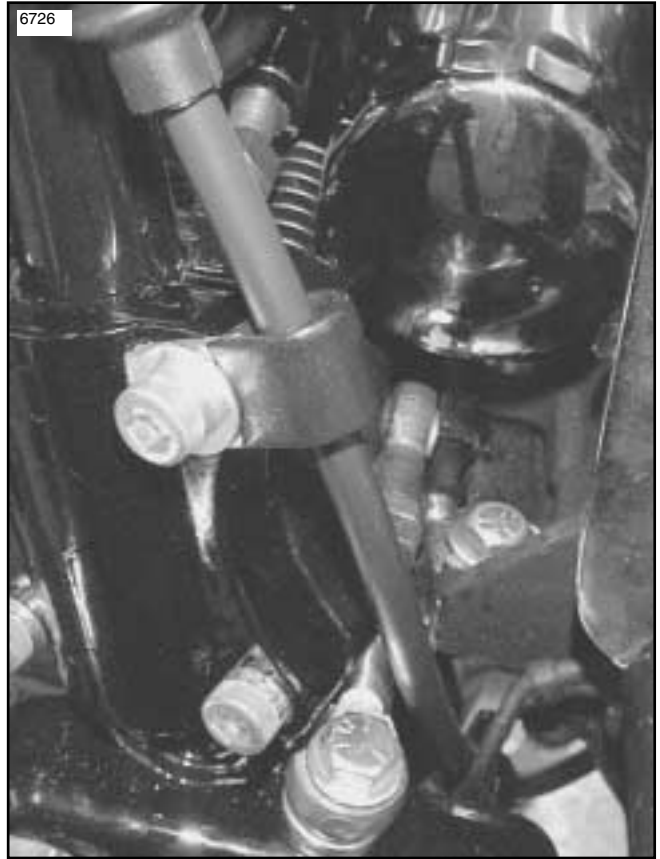
Figure 2. Clutch Cable Routing (Behind Regulator)
