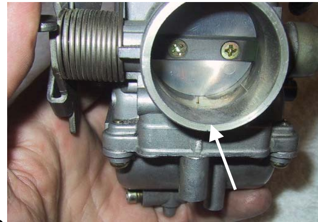
At 6 o'clock in the mouth of the carb you can see the end of the idle mixture needle poking up. Engine Side, Butterfly Closed
