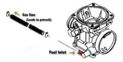
Going a little farther, Stage I: Shut off fuel petcock. Drain carburetor into container. Remove fuel line at carburetor input. I nsert carburetor cleaner spray can nozzle into carburetor fuel inlet port. Spray the Dickens out of that sucker, until pure carb cleaner flows into container. Reconnect the fuel line and cycle the float bowl with gasoline as before; shut the drain screw and giver 'er a try.
