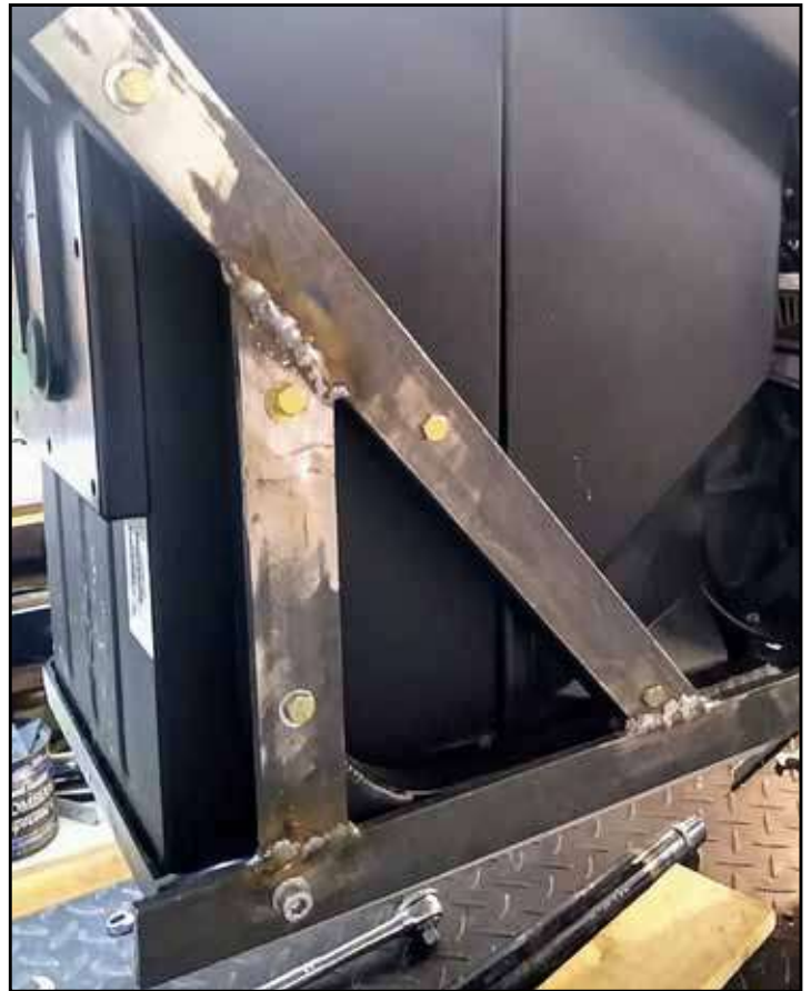
Both side fabrications fitted and welded up. Now I'll make a bolt on front cross member.
