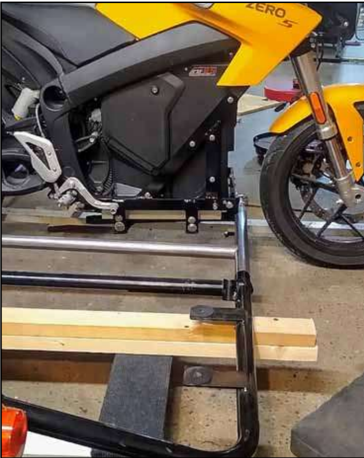
When I set the toe-in I found my front arm would hit the subframe.
